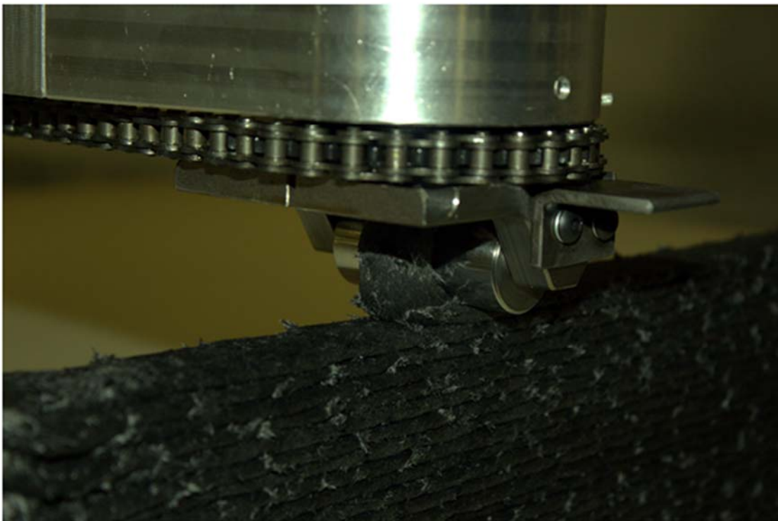
Thermwood's MeltShape wheel is servo controlled to precisely follow machine motion
